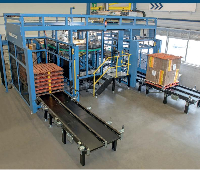
The **Buhrs DPS** is a revolutionary system for the automatic depalletizing of pallets with flat packaging. The starting points for this new system – developed by Buhrs – were high net output, maximum automation, reduction of human touch points and minimization of the transport movements around the machine.
